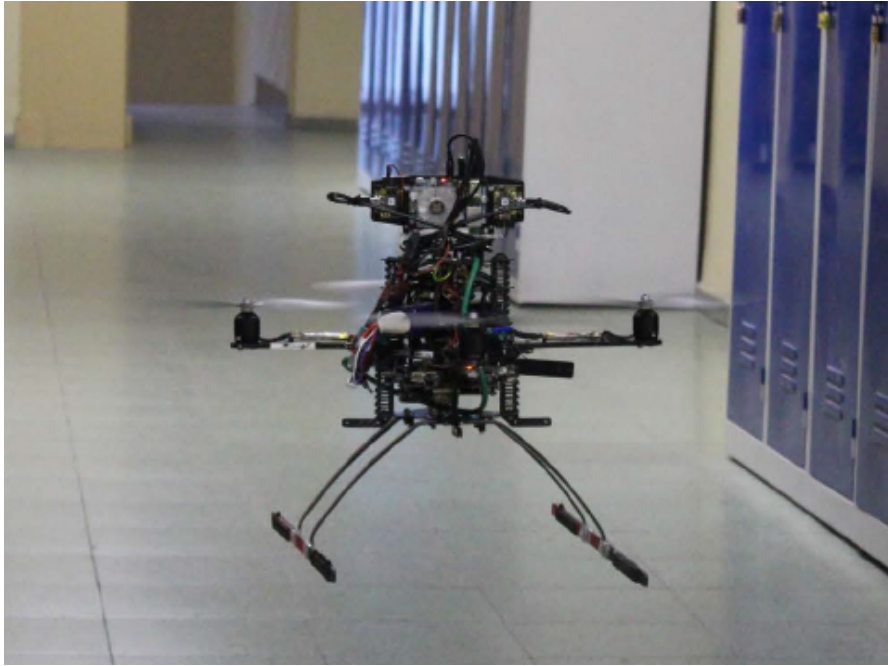
Figure 1.1: Quadrotor UAV with Stereo Camera Flying Indoor. This image shows a quadrotor UAV with a stereo camera mounted on its top for indoor navigation. Since the robot operates inside of a building, no GNSS signals can be received. Instead, the UAV navigates using the stereo camera.
